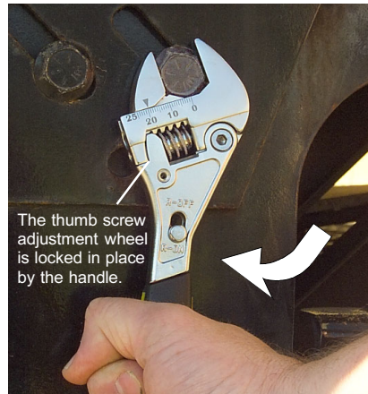
Pivoting the handle upward releases the adjustment wheel allowing jaws to open slightly and ratchet around the bolt head.
