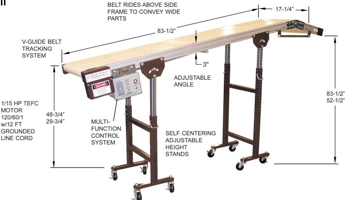
The PPE FTP Conveyor is ideal for use where your parts picker drop off is high in the air. The picker can gently place your parts on the conveyor where they are conveyed down to operator height for manual or automated removal from the conveyor. The On/Off cycle timer helps avoid unnecessary wear and tear on the belt by not running it continuously and also prevents the Lucille Ball effect where the operator cannot keep up with the conveyor.
