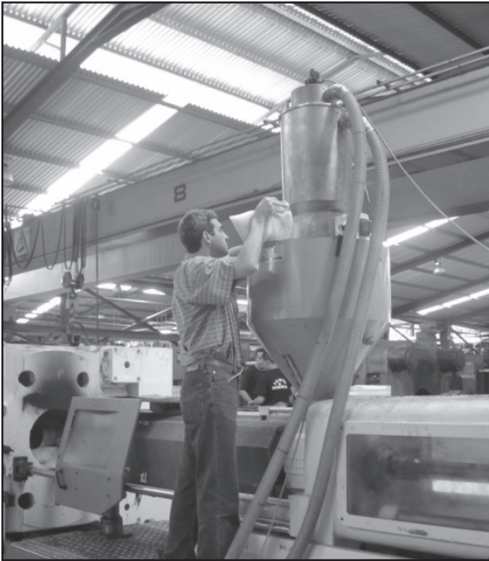
Mix only 10% EPC Concentrate with 90% virgin resin.
