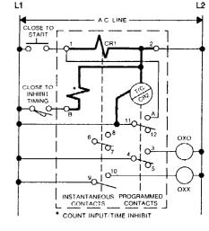
Standard Start — Close start switch to time; open to reset. Cycle progress is stopped without reset by closing inhibit switch. Unit resets on power failure. Setpoint is maintained by battery. Instantaneous contacts actuate with start switch. The programmed contacts actuate as programmed by rocker switches 3-5.
