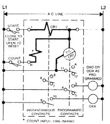
Standard Start — Close start switch to start, open to reset. Counts are registered when count switch opens. Unit resets on power failure. Setpoint is maintained.
