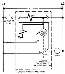
Momentary or Sustained Start — Close to time. Automatic reset at end of timing period with start switch open or closed. (Programmed for OXO output ONLY.)
