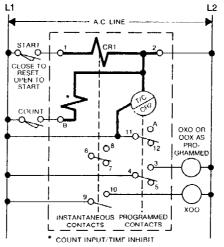
Reverse Start — Close start switch to reset, open to start. Unit does not reset on power failure. Battery retains cycle progress and setpoint
