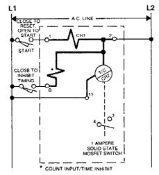
Reverse Start — Open switch to time; close to reset. Cycle progress is stopped without reset by closing inhibit switch. Unit does not reset on power failure. Battery retains cycle progress and setpoint.
