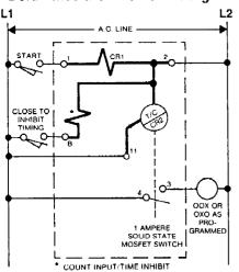
Standard Start — Close start switch to time; open to reset. Cycle progress is stopped without reset by closing inhibit switch. Unit resets on power failure. Setpoint is maintained by battery. Solid state delay contact actuates as interval (OXO) or delay (OOX) sequence as programmed by rocker switches.
