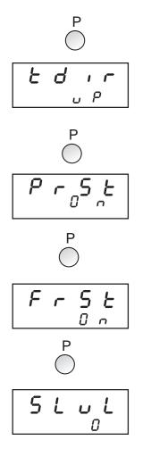
**Timing Direction:** Determines whether the time value will increment from zero and change the state of the output at the set value (uP) or decrement from the set value and change the state of the output at zero (dn).
