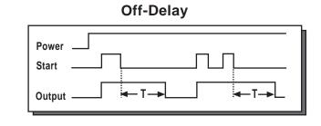
The output is activated at the leading edge of the start signal. Timing begins on the trailing edge. The output will remain active until the preset time (T) has elapsed or power is interrupted\*. Reapplying the start signal before T has elapsed will reset the time value. The reset input is not used.
