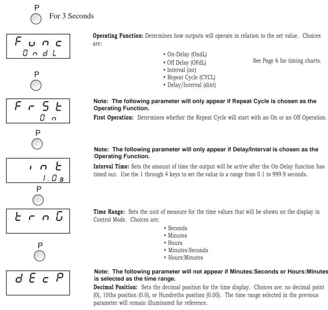
**Operating Function:** Determines how outputs will operate in relation to the set value. Choices are:
