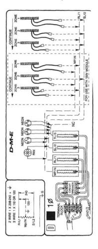
The diagram to the left depicts two different wiring configurations. One is 208-240 volt, single-phase, 3-wire. Note that lines RL1 and SL2 are connected through the circuit breaker to the appropriate terminal strips. All modules in this system will be connected between RL1 and SL2. MP/N is common with ground and is not connected through the circuit breaker.
