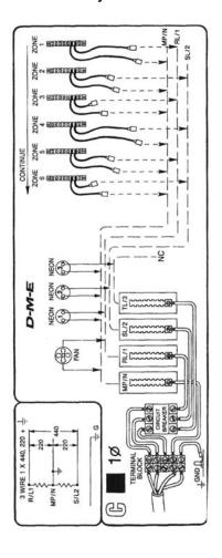
The 240 volt single-phase connection only uses two power lines plus ground.
