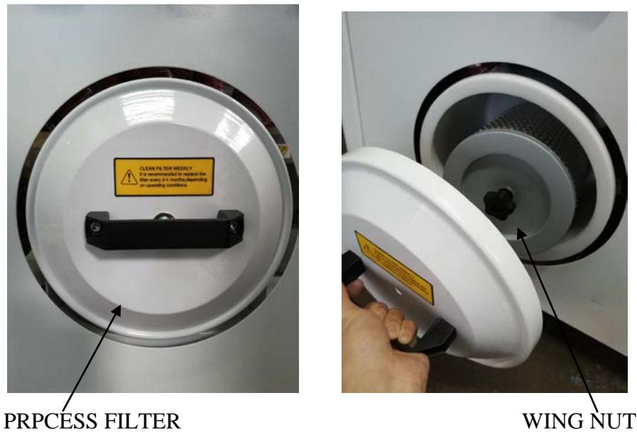
**Figure 4-5. Process Filter Replacement**
