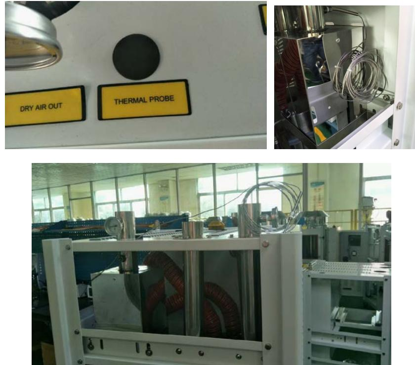
Figure 3-5. Thermal probe for connecting hopper dryer
