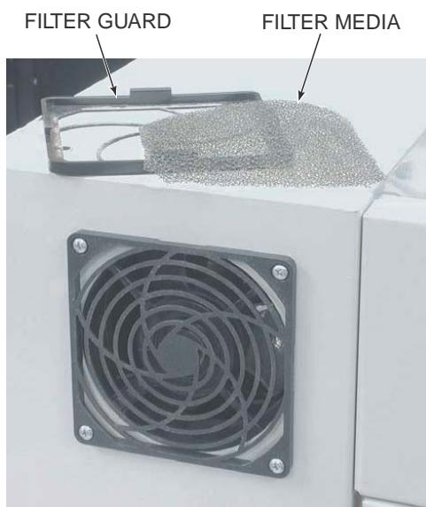
**Figure 4-6. Control Box Filter Replacement**
