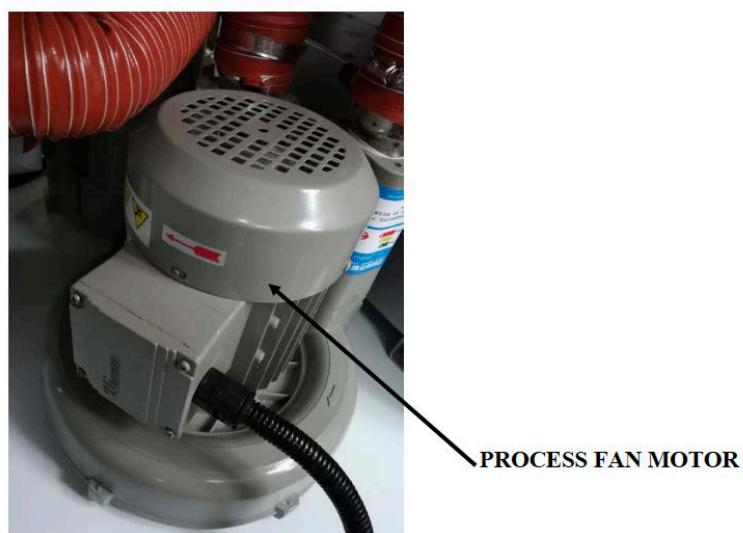
**Figure 3-1. Process Fan Motor**
