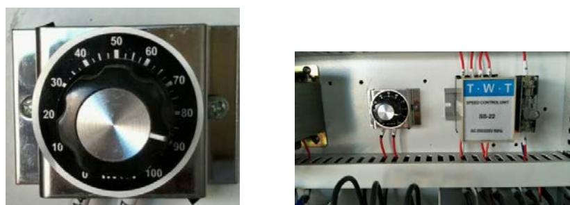
Figure 3-4. Adjusting gadget for desiccant rotor speed
