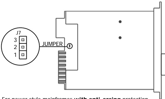
Pin 1 & 2 - For newer style mainframes **with anti-arcing** protection.
