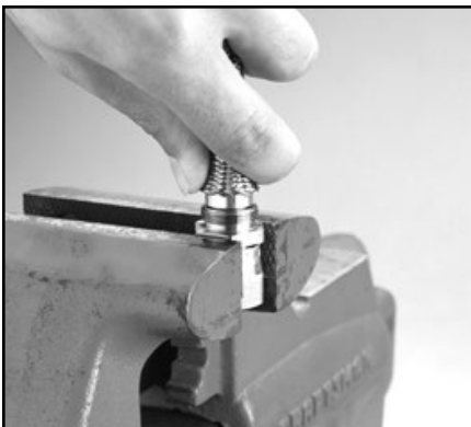
12. Using a twisting motion, push hose over nipple until hose is seated against nipple chamfer.
