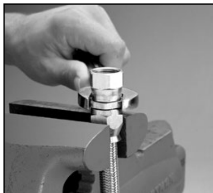
16. Tighten further to align corners of nipple and socket hexes if necessary. Repeat Steps 4 through 16 for other end of hose.
