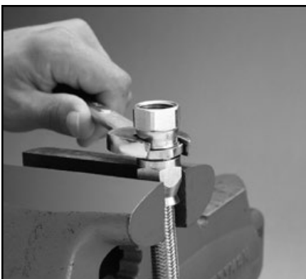
15. Wrench tighten nipple hex until clearance between hex and socket hex is 1/32" or less.
