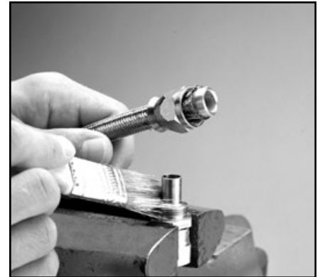
11. Using SAE 20 weight lubricating oil, lubricate nipple and socket threads. For stainless steel fittings use Parker ThreadMate™ or a molybdenum type lubricant. For hose used in oxygen service lubricate using a non-oil based soap solution.
