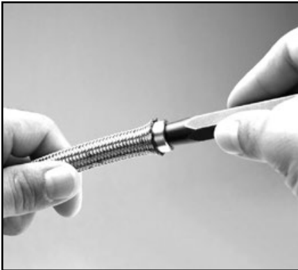
10. Using a tapered punch, push punch into end of sleeve and tube to set sleeve barbs into tube.
