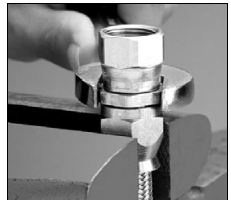
14. Remove assembly from vise and reposition with socket in vise jaws. Ensure socket extends beyond vise jaws far enough to allow nipple to be completely tightened.
