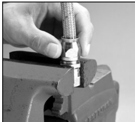
13. Push socket forward and hand-start threading of socket to nipple. Caution: When tightening socket in vise, do not over tighten vise jaws. Over tightening vise jaws will distort internal threads of socket.
