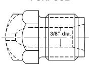
For use on General Purpose Materials such as Polyethylene, Styrenes, etc.
