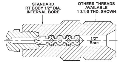
Illustrated: Standard Removable Tip RT Nozzle Body Model R-1 Style A 5" Length O.A. (with tip in place), 1 3/4-8 thread, 3/4" rear opening can be converted to color mixing pineapple type by adding Conversion Tip Model RTP.
