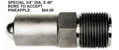
Illustrated: Solid Nozzle Model R-1D5, Pineapple Dispersion Nozzle, 5" length overall, 1 3/4-8 thread, 3/4" rear opening bored with a 3/4" dia. x 40° angle internal hole to accept a 3/4" dia. pineapple.
