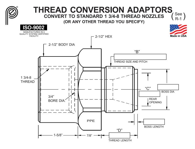
ALWAYS USE A THREAD LUBE! EXAMPLE: CONVERT A METRIC THREAD TO A STANDARD 1 3/4-8 FRONT THREAD
