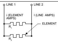
PARALLEL One or more elements wired across two line wires. Element volts equal line volts. Total power is equal to sum of watts in each element. Line amps equal sum of current of each
