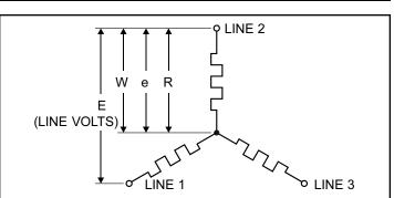
**STAR or WYE (3Ø)** Three elements or group of elements wired in a Wye ("Y"). Total power is  $W = 1.73E \times I$ , where E is volts between any 2 lines and I is current in any 1 line. Volts across each element (volts to neutral) is e = E/1.73. Current thru each element is same as each line wire.
