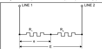
SERIES Two or more elements or equal resistance wired together and across line wires. Element volts equal line volts divided by number of elements. Total power is equal to sum of watts of elements. Line amps equal current thru each element.
