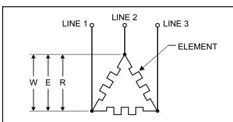
**DELTA (3Ø)** Three elements or groups of elements wired in a triangle (Delta). Power is: W = 1.73E x I where E is volts between any 2 lines and I is current in any 1 line. Power in each side of Delta is 1/3 of total. Volts across each element is full line volts. Current thru each element is i = E/R.
