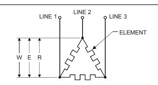
**DELTA (3Ø)** Three elements or groups of elements wired in a triangle (Delta). Power is:  $W = 1.73E \times I$  where E is volts between any 2 lines and I is current in any 1 line. Power in each side of Delta is 1/3 of total. Volts across each element is full line volts. Current thru each element is i = E/R.
