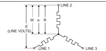
**STAR or WYE (3Ø)** Three elements or group of elements wired in a Wye ("Y"). Total power is  $W = 1.73E \times I$ , where E is volts between any 2 lines and I is current in any 1 line. Volts across each element (volts to neutral) is e = E/1.73. Current thru each element is same as each line wire.
