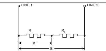
**SERIES** Two or more elements or equal resistance wired together and across line wires. Element volts equal line volts divided by number of elements. Total power is equal to sum of watts of elements. Line amps equal current thru each element.
