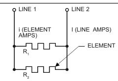
**PARALLEL** One or more elements wired across two line wires. Element volts equal line volts. Total power is equal to sum of watts in each element. Line amps equal sum of current of each element.
