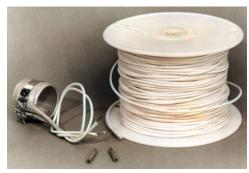
1. Select wire size to suit your amperage requirements. Normally size 18 TGGT 600 volt wire is used on nozzle bands. It can carry a load of 2760 watts on 120 volt or 5520 on 240 volt.
