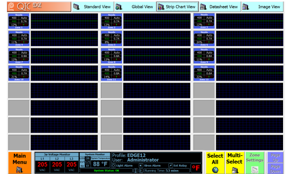
Graph View: View real-time graphs for up to 24 zones at a time.
