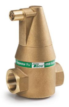
The Taco® 4900 Series Air Separators are designed for the complete elimination of air from closed loop heating and cooling systems up to a maximum temperature of 240°F and a maximum pressure of 150 psi. The principle on which the 4900 Series Air Separators operate is a patented and proven method of removing gases from water called the PALL ring process.
