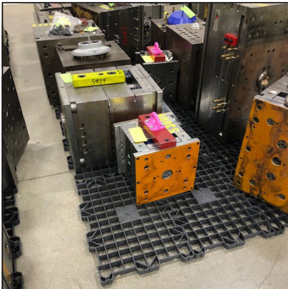
Mold Mats used for long term mold storage.
