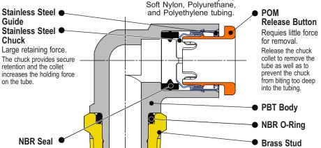
Can be used for a wide range of pressures from low vacuum up to 145 psi. The use of a special profile ensures sealing and reduces resistance when the tube is inserted
