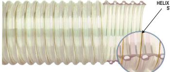
PROTECTED COPPER STATIC **GROUND WIRE RUNS NEXT TO** HELIX OF HOSE FOR POSITIVE STATIC DISSIPATION
