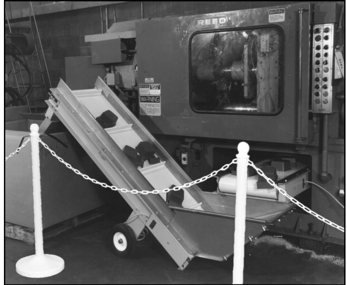
STANCHIONS CAN BE USED TO GUIDE PERSONNEL AROUND MACHINERY IN OPERATION.
