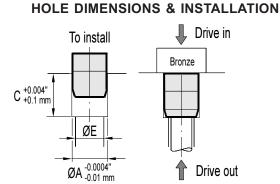
Drill a hole per the specifications listed. Insert has an undersized portion to allow partial entry into the drilled hole. Use a bronze block against the insert face and drive down into position. To remove, drive out from the
