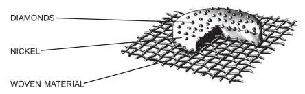
CROSS SECTION REVEALS UNIQUE CONSTRUCTION OF HARD NICKEL ISLANDS ELECTROPLATED THROUGH BASE MATERIAL TO GRIP & HOLD DIAMOND CRYSTALS.
