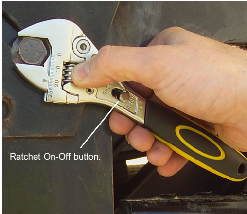
The thumb screw adjustment wheel is locked in place by the handle.
