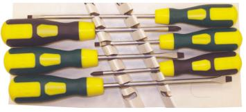
NOTE: Cabnet Tip blade is same width as shaft for deep holes.
