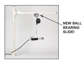
The WS-2000 is a complete ergonomic support system for use with any power pack and jaw set combination in our product line. This heavy duty work station features a 36" horizontal, 180° boom attached to a 48" vertical column with a base that mounts easily to bench tops. The boom can be adjusted vertically higher or lower on the column to suit your specific application.
