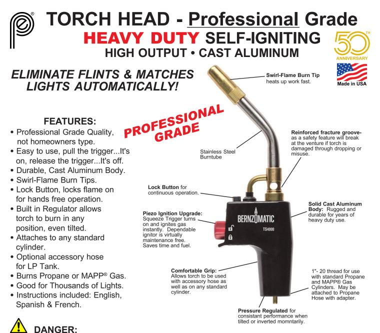
**TS4000 Brazing Self-Igniting High Output Cast Aluminum Torch**, pull the trigger it's on, release the trigger it's off. Locking button keeps flame on continuously if needed. Burns propane or the much hotter MAPP<sup>®</sup> gas for difficult tasks. Stainless steel burntube, cast aluminum body and swirl-flame burntip for durability.
