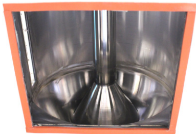
Stainless Steel internal air pipes & dispersion cone.
