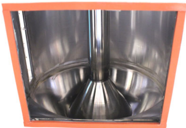
Stainless Steel internal air pipes & dispersion cone.
