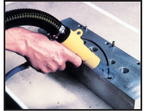
Cleaning chips out of a fixture base is one of the numerous uses for the deep hole air gun.
