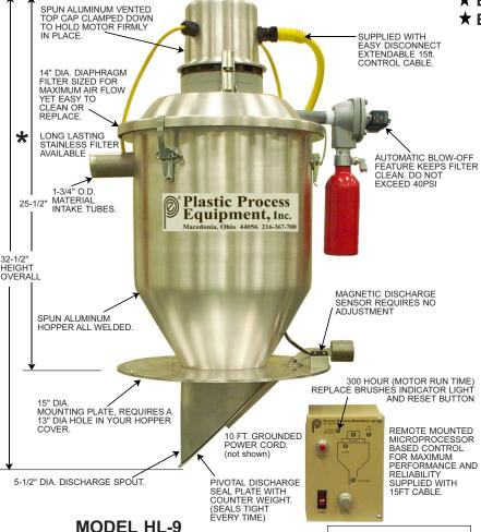
To reduce dangerous static electricity, connect the ground wire between your hopper loader and the metal pickup probe in your material supply. PPE Loaders are supplied with vacuum hose that includes a static ground wire.
