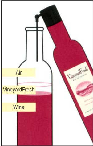
How VineyardFresh works with unique spray-through cap and hinged extension tube.
